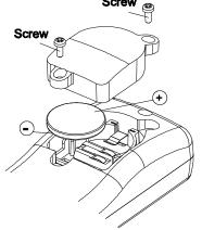
Battery Compartment Cover Battery Replacement
